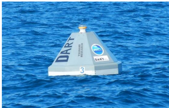
Figure 9-6 Deep-Ocean Assessment and Reporting of Tsunamis System (DART)
